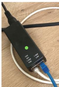
Locate the **PoE** which is the little black box that supplies power to the outside radio/antenna. This PoE has a power cord, two ethernet cables and a glowing light when power is connected.
